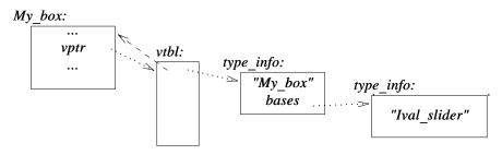
The dashed arrow represents an offset that allows the start of the complete object to be found given only a pointer to a polymorphic sub-object. It is clear that *dynamic\_cast* can be efficiently implemented. All that is involved are a few comparisons of *type\_info* objects representing base classes; no expensive lookups or string comparisons are needed.
