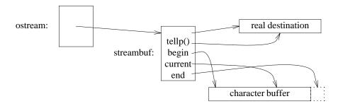
The set of template arguments for an *ostream* and its *streambuf* must be the same and determines the type of character used in the character buffer.
