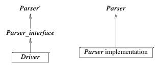
To ensure the consistency of *Parser* and *Parser*<sup>'</sup>, we again rely on the compilation system as a whole, rather than on just the compiler working on a single compilation unit. This solution differs from the one in §8.2.4 only by the extra namespace *Parser\_interface*. If we wanted to, we could give *Parser\_interface* a concrete representation by giving it its own *expr()* function:
