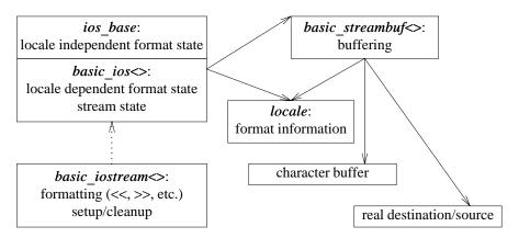
The dotted arrow from *basic\_iostream*<> indicates that *basic\_ios*<> is a virtual base class; the solid arrows represent pointers. The classes marked with <> are templates parameterized by a character type and containing a *locale*.
