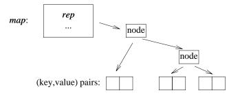
A map is most likely implemented as a (balanced) tree of nodes pointing to (key,value) pairs:
