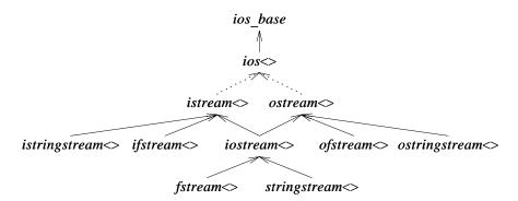
The classes suffixed by  $\langle \rangle$  are templates parameterized on the character type, and their names have a *basic* prefix. A dotted line indicates a virtual base class (§15.2.4).
