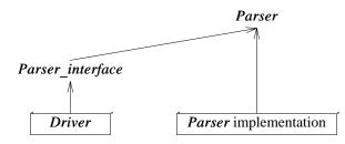
Now the *driver* appears vulnerable to any change in the *Parser* interface from which it was supposed to be insulated. Even this appearance of a dependency is undesirable, so we explicitly restrict *Parser\_interface*'s dependency on *Parser* by having only the relevant part of the implementer interface to parser (that was called *Parser'* earlier) in scope where we define *Parser\_interface*:
