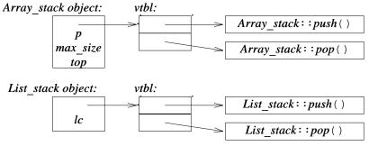
The functions in the *vtbl* allow the object to be used correctly even when the size of the object and the layout of its data are unknown to the caller. All the caller needs to know is the location of the *vtbl* in a *Stack* and the index used for each virtual function. This virtual call mechanism can be made essentially as efficient as the ''normal function call'' mechanism. Its space overhead is one pointer in each object of a class with virtual functions plus one *vtbl* for each such class.
